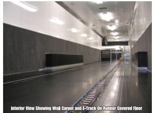
Interior View Showing Wall Carpet and E-Track On Rubber Covered Floor
